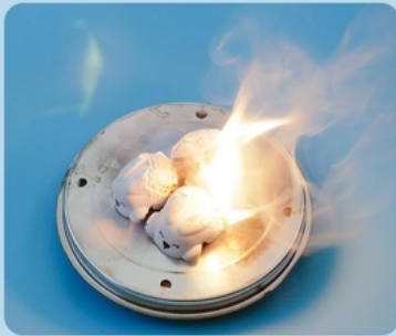
Silicone burning produces white smoke
