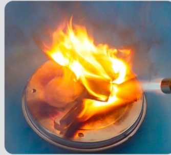
PVC/Rubber burning produces black smoke
