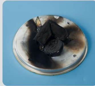
PVC/Rubber burning produces black smoke
